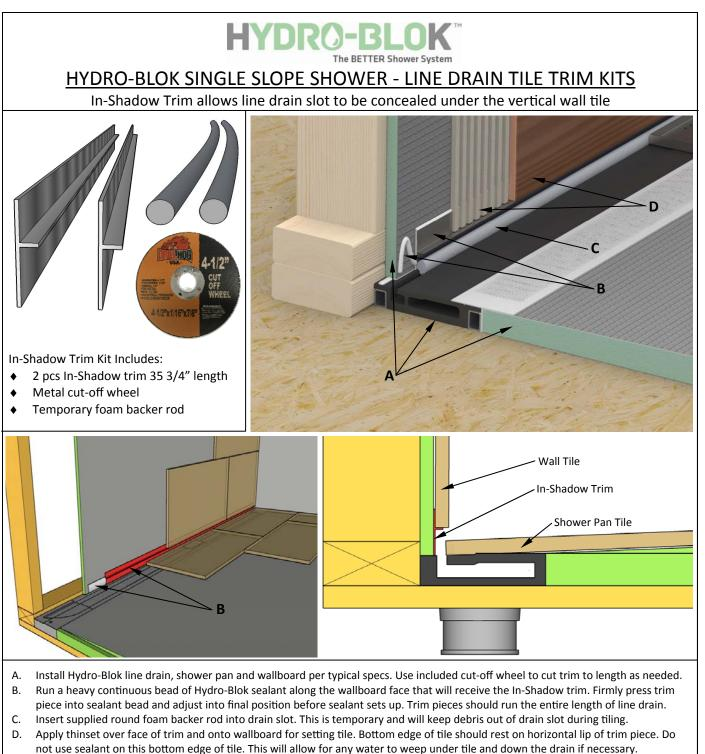
\*\* PLEASE NOTE: In-Shadow trim can be used with 1/4" - 3/8" shower pan tile. When cutting trim to desired length it is best practice to place all cut edges at the outer ends of line drain. This will allow factory edges to be butted together when using multiple trim pieces. Trim pieces are made from high quality 304 Stainless Steel .25mm thick
